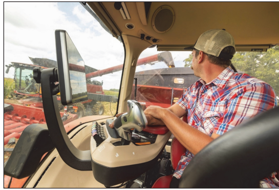
Figure 11. Photograph from front of tractor of grain cart operator (not study participant) during stationary unload event. Using RCA, the operator can continually look back at the combine and the grain cart but does not hold the steering wheel (bottom right) because RCA controls steering and matches the combine's speed.
