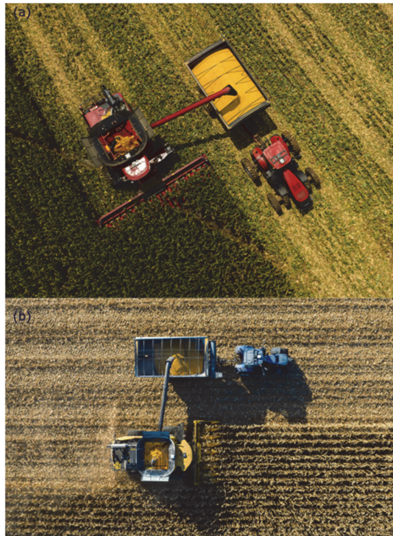
Figure 2. Aerial photographs of representative on-the-go unload events in corn with (a) Case IH 8250 and Magnum 310 and (b) New Holland CR8.90 and T8.
