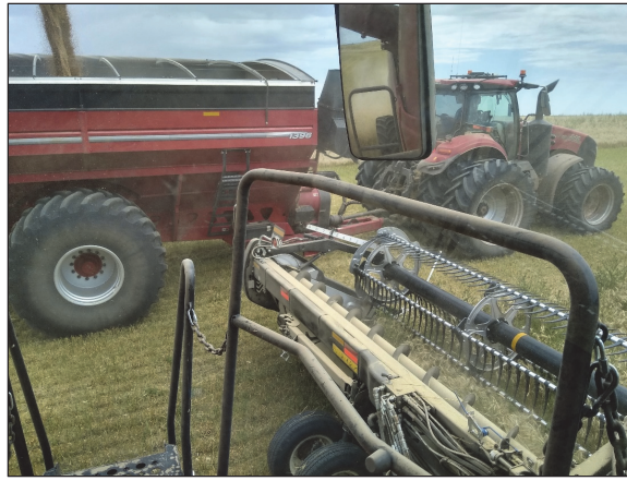
Figure 1. Photograph from the combine of an on-the-go unload event in wheat. Note the close proximity of the grain cart to the combine header.
